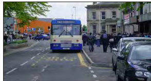
Photo 71 – Full width bus boarder
